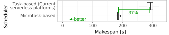
Fig. 1. Exemplary result comparing the makespan of serverless sort implementation with microtask-based scheduling to one with task-based scheduling. The microtask-scheduling based version finishes 37% earlier, by median values.
